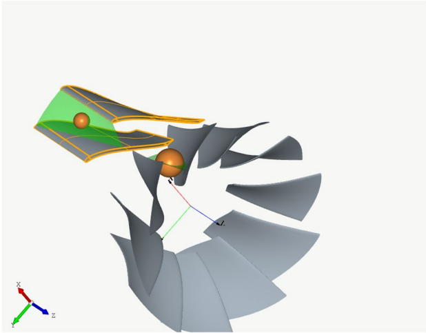
Fig. 12 The 3D geometry of the Francis turbine and the flow passage area in the IGV
